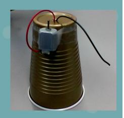
You tape the vibrating motor with wires to the top of the cup.
