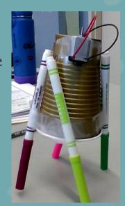
You put the eraser to the vibrating motor to the top of the cup.
